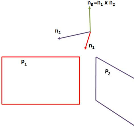
Fig. 1. Construction of 3D rotational frame from two non parallel planes,  $P_1$  and  $P_2$  using their respective normal vectors  $n_1$  and  $n_2$ . Third normal  $n_3$  is computed by the vector cross product between the two normals.
