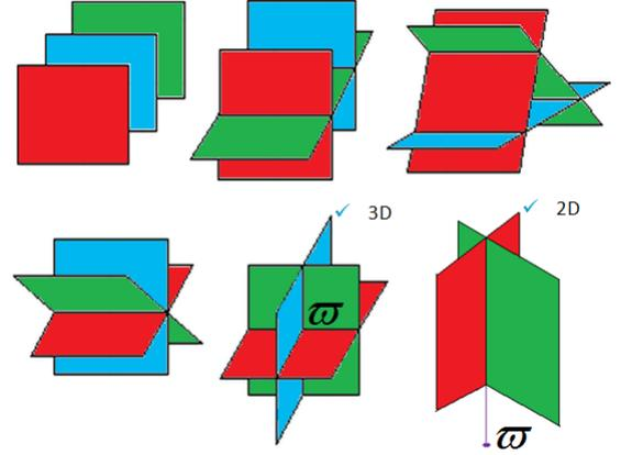
Fig. 2. Construction of 3D rotational frame from two non parallel planes,  $P_1$  and  $P_2$  using their respective normal vectors  $n_1$  and  $n_2$ . Third normal  $n_3$  is computed by the vector cross product between the two normals.
