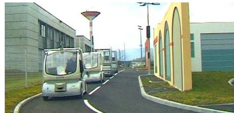
Fig. 1. Experimental vehicles: a Cycab leading three Cycab/RobuCab
